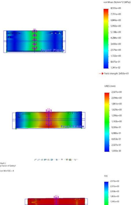
Model name: Tabletop Study name: Static 1(-Default-) Plot type: Factor of Safety Factor of Safety1 Criterion : Automatic Factor of safety distribution: Min FOS = 4
