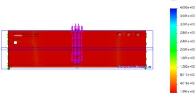
The maximum displacement is now 5 mmm, which is too much. The safety factor is now just a little bit less than 2, namely 1,991. The desk would still be strong enough to carry the weight of one person, given that the safety still has a value of about 2. The displacement is higher than it should be though.
