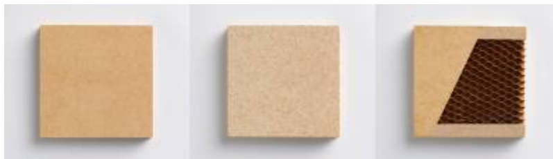
Figure 24: Honeycomb Structure in Ikea Furniture
